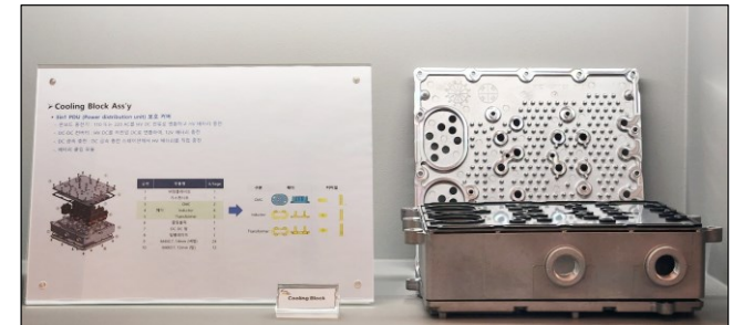
Cooling Block & PDU
